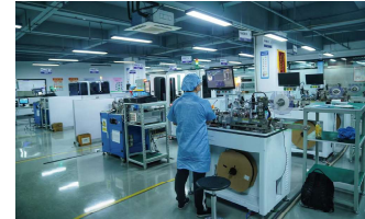
100% Visual Inspection and Withstand Voltage Test
