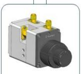
VAB3101SF\* Frequency: DC - 2.7 GHz Power Rating: 2W or 5W Attenuation: 0 - 31 dB Step Value: 1 dB Insertion loss: <0.5 dB Attenuation Accuracy:  $\pm 0.6$ dB VSWR:  $\leq 1.25$ Size: 32\*39\*80mm Mass production has been arranged; 40%-50% price lower than other manufacturers'.
