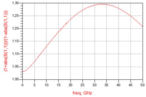
Test result of add 300um double wire-bonding
