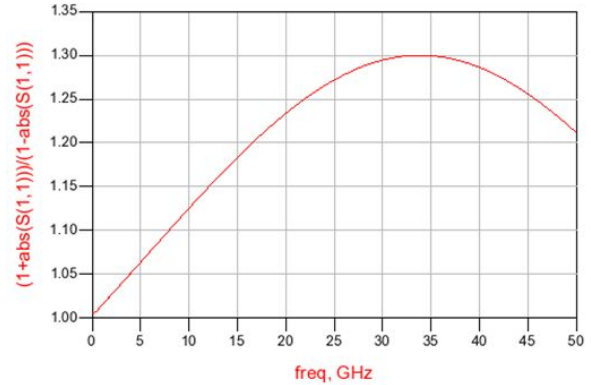
Test result of add 300um double wire-bonding
