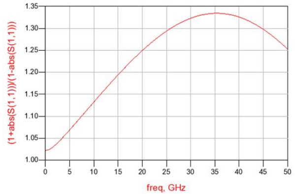
Test result of add 300um double wire-bonding
