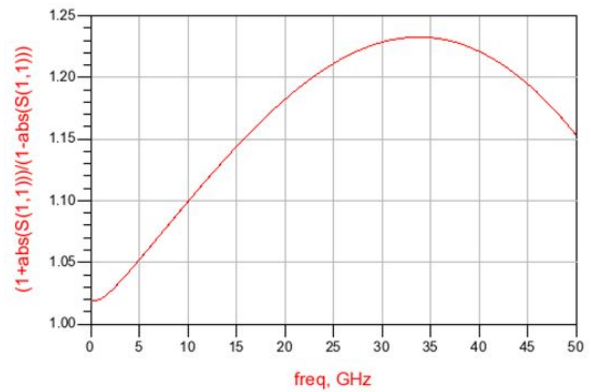
Test result of add 300um double wire-bonding
