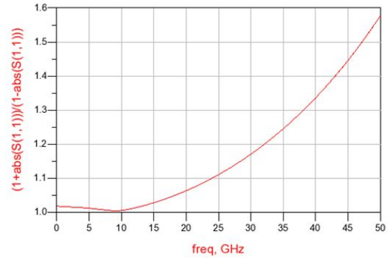
Test result of add 300um double wire-bonding
