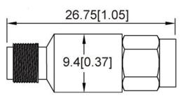
Package type: SMA Note: all dimensions shown in mm & inch
