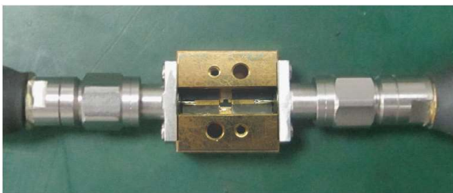
Connect test part to Test Fixture
