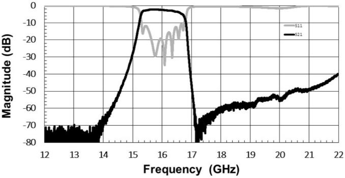
\*Typical de-embedded measured performance mounted on a connectorized test fixture. DEB is 0.254mm RO4350B with 50.00hm CPW ground traces going into the ports at room temperature.
