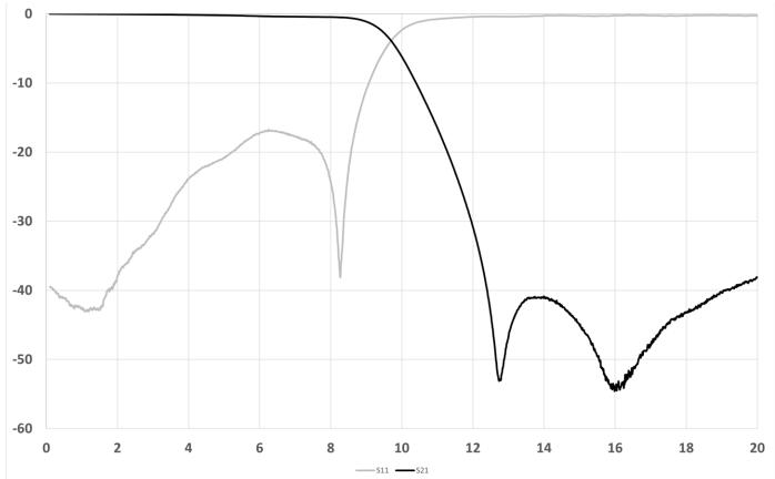
\*Typical de-embedded measured performance mounted on a connectorized test fixture. DEB is 0.254mm RO4350B with 50.00hm CPW ground traces going into the ports at room temperature.
