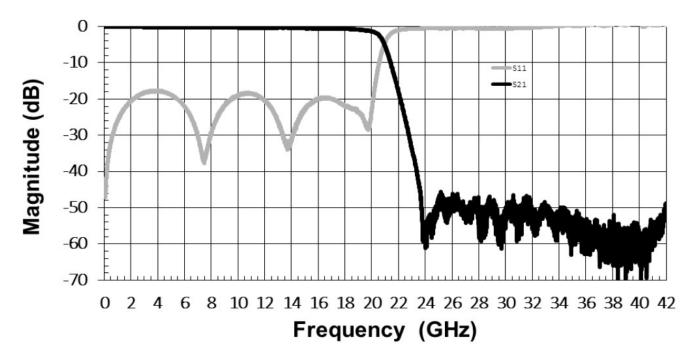
\*Typical de-embedded measured performance mounted on a connectorized test fixture. DEB is 0.254mm RO4350B with 50.00hm CPW ground traces going into the ports at room temperature.
