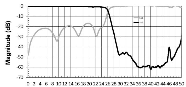
\*Typical de-embedded measured performance mounted on a connectorized test fixture. DEB is 0.254mm RO4350B with 50.00hm CPW ground traces going into the ports at room temperature.
