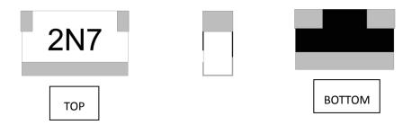
=: Effective drawing shows as below after completion of part soldering, soldering will be done with the contact of bottom side and microstrp line, silkprint mark must be upwards in order to identify the part number and specification. It may have influence on the part reliability if not use part with correct soldering in comply with operation instruction.
