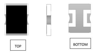
=: Effective drawing shows as below after completion of part soldering, soldering will be done with the contact of bottom side and microstrp line, black isulating resin must be upwards. It may have influence on the part reliability if not use part with correct soldering in comply with operation instruction.
