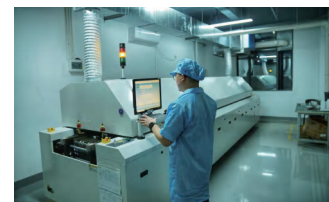
Reflow Welding Test in 10 Temperature Zone
